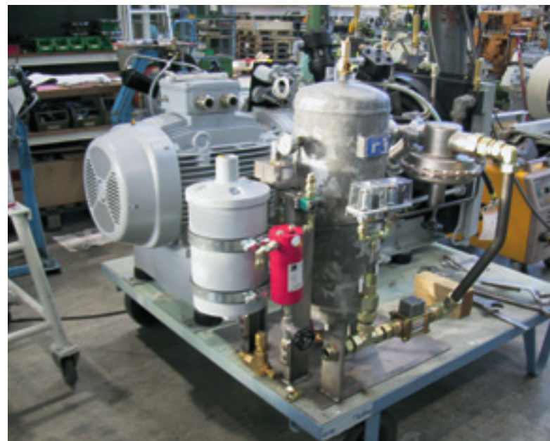
Using PSA gas generator and WP 4331 high-pressure 'H' series compressor
